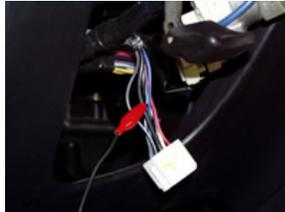
This is another picture of the IGNITION SWITCH Harness Plug removed for the Ignition switch of the vehicle.
