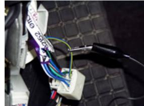
The (TYPE B) BLUE/YELLOW UNLOCK wire, marked with the BLACK Clip, is located in this WHITE Plug, in the DRIVERS KICK PANEL.
