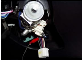
This shows the IGNITION HARNESS unplugged from the IGNITION Switch to expose the IGNITION wires for IDENTIFICATION.
